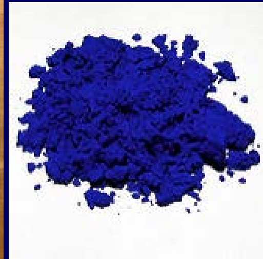
Synthetic ultramarine pigment is chemically identical to natural ultramarine
