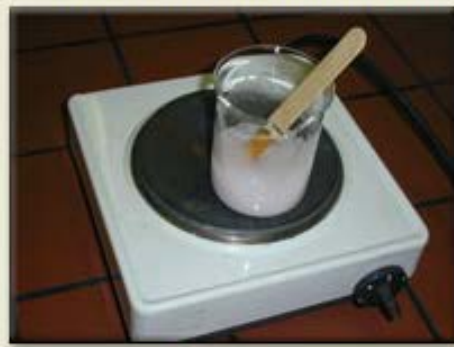
alizarin is added to the aluminum hydroxide
