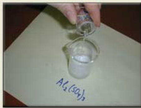
The solution of sodium carbonate is poured into the solution of aluminum sulfate
